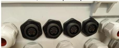
Figure 63 – 4 prises Modbus IP67
