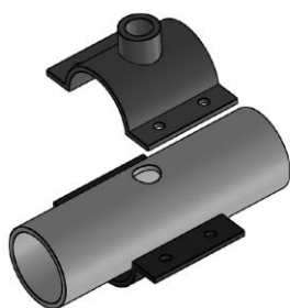
Figure 79 – Drill Hole Ø 20mm (3/4")
