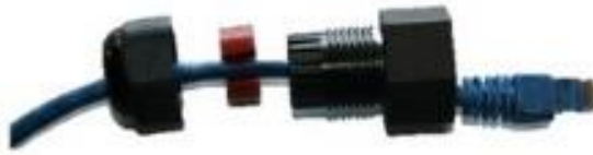
Figure 86 - RJ45 Connector for Ethernet
