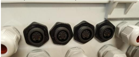
Figure 65 – Four Modbus IP67 sockets.
