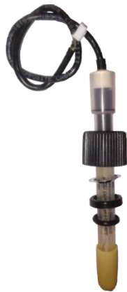
Figure 45 -Water Analysis Sensor with Transport Cap
