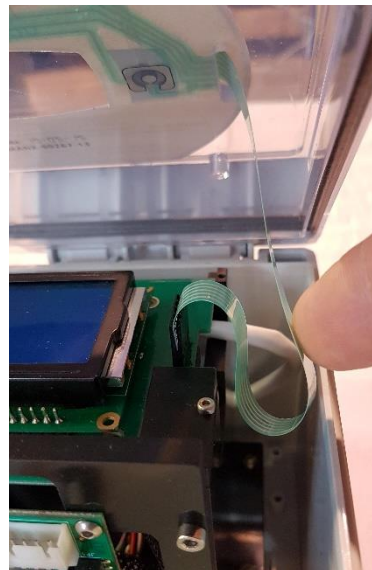
Figure 35 - Guide Ribbon Cable into the Enclosure
