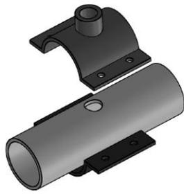
Figure 79 – Perçage Ø 20mm (3/4")
