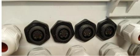
Figura 65 – 4 soquetes Modbus IP67
